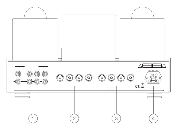
1) Signal input: Inputs (RCA plugs) are for connecting a «line level» source to your amplifier. It is designed to receive an «analog» signal (as opposed to «digital» signal). To connect your source we are using a traditional «RCA» cable, they are usually identified by a color code «RED» to the RIGHT channel and «WHITE» to the LEFT channel.
